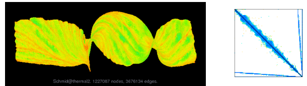
Fig. 6. Left : For the unstructured FEM, steady state thermal problem, this graphic visualization is provided by [42], [43]. Right : The sparsity pattern for this system.
